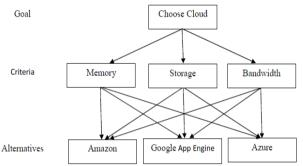
Figure 2: Application of AHP for the selection of functional requirements
